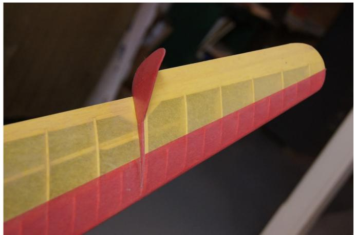
Here is a picture of someone who built the original 50inch (I suspect a free flight) version, and what you see here is that the (inboard) rudder is pointing outwards. I think just on one side to get the glider flying in a circle. Nicely built though.
